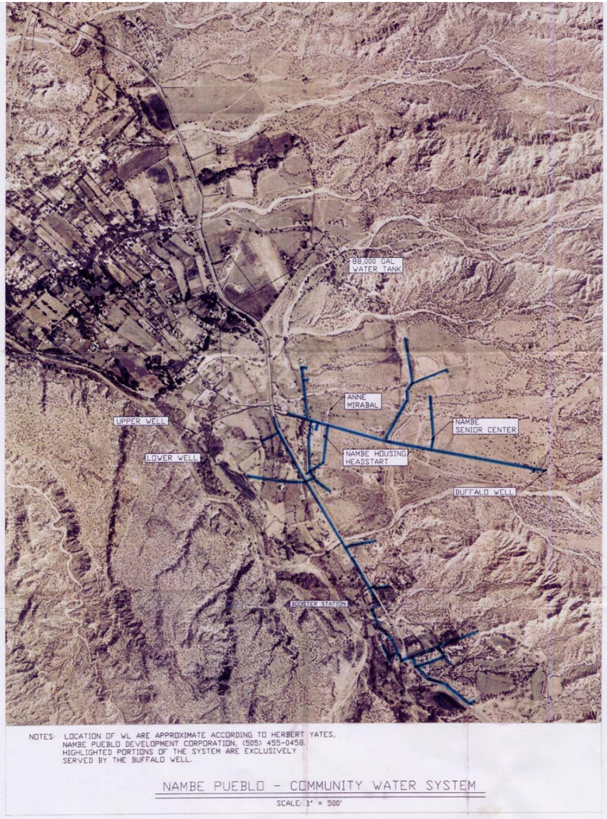
Figure 4-5. Nambe Pueblo Water Distribution System Map
